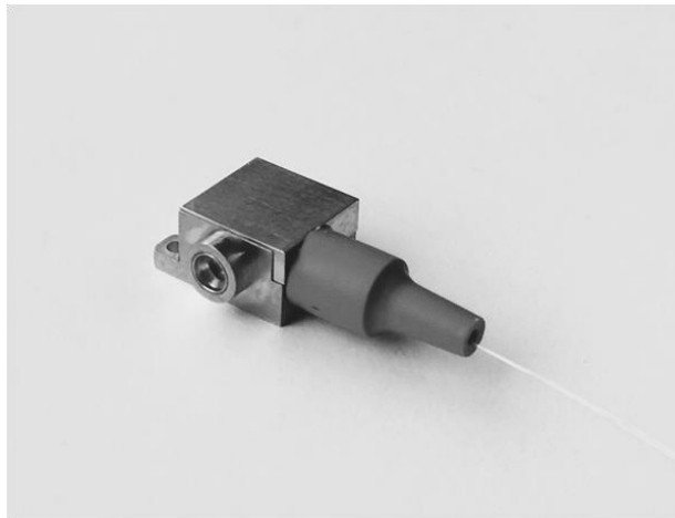
Figure 5. Photograph of Freedom Photonics' packaged MUTC photodetector, with the lowest package volume (1.3 \text{cm}^3 ) and an integrated bias-tee.
