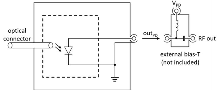
Block diagram of FP1015a. An external bias-T of  $\geq 30$  GHz (-3-dB) is required.
